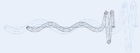
Helical bird flight diverter for all earth wires and overhead lines
