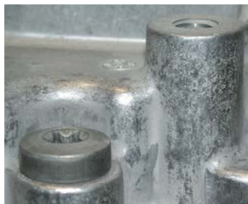
RIBE-Aluform® magnesium housing connection before and after a 24-h salt spray test
