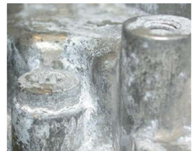
RIBE-Aluform® magnesium housing connection before and after a 24-h salt spray test
